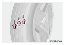
Check the tire tread by the tread wear mark. When tread wear reaches its limit, tread will be in the same plane as the wear band. At this time, it indicates that performance and safety of tire seriously decrease, and replacement is necessary.
