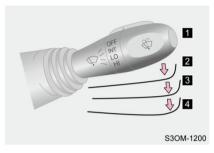
Turn power switch to ON, move wiper combination switch:
