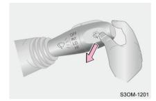
Turn power switch to ON, pull wiper combination switch towards steering wheel and hold, the front washer sprays water, and front wiper operates simultaneously. Front washer will stop operating when the switch is released, the wiper will wipe 3 cycles at low speed.
