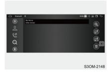
When Bluetooth is not connected, click to enter the Bluetooth setting interface; when Bluetooth is connected, click to enter the dialing interface.
