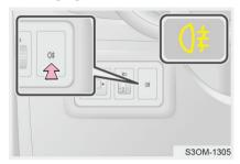
When the low beam lights of headlight are on, press rear fog light switch on the instrument panel switch to turn on rear fog light, rear fog indicator on instrument cluster will come on.
