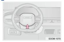
To sound the horn, press center area of the steering wheel.
