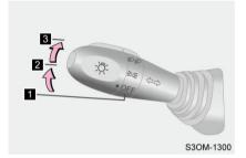
Turn power switch to ON, rotate headlight combination switch:
