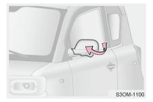
Push the rear view mirror forwards or backwards to fold outside rear view mirror.
