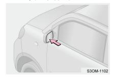
Press the edge of lens by hand to adjust to a suitable visual field.
