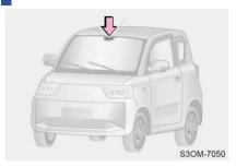
The microwave window is located on the inner side of the front windshield and at the right side to the back of the inside rear view mirror, where is for wireless RF signal transmission and installation of automotive electronic identification.
