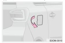
Step 2: Pull the protruding area on edge of charging port cover to open the charging port cover.
