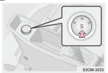
Press the driving mode button S (ECO mode by default) on the shift switch to switch between ECO mode and SPORT mode. When S indicator comes on, it is in SPORT mode; When S indicator goes off, it is in ECO mode. The motor speed will be reduced in ECO mode, improving the vehicle power economy. At this time, the maximum speed limit is 70 km/h.
