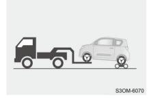
Place towing dolly under rear wheels. **Never towing with sling-type truck**
