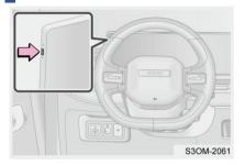
The adjusting button can be used to switch the display mode and reset the trip mileage, and is located on the left side of dual screen. Shortly press once to switch one page, there are 3 pages in total. It can display voltage, current. motor speed. motor temperature. average power consumption, trip mileage and DTC display, etc. To reset the trip mileage, long press the adjustment button for more than 3 seconds in trip mileage display interface on the second page.
