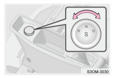
Depress brake pedal, and lightly turn shift knob to switch to required gear position. Current gear position is displayed on instrument cluster. The corresponding gear position indicator on knob also comes on.
