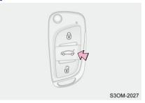
Long press back door opener button on remote control key for 2 seconds and back door will be unlocked.
