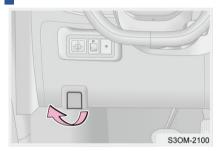
Step 1: The front compartment cover will pop up slightly by pulling front compartment cover opening handle on the lower left side of the instrument panel.
