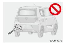
High pressure water flow such as water guns or large external forces may damage the radar sensors. Do not pinch or impact the radar sensors, otherwise the sensors will not work normally.
